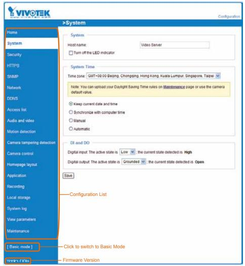
Each function on the configuration list will be explained in the following sections. Those functions that are displayed only in Advanced Mode are marked with Advanced Mode. If you want to set up advanced functions, please click [Advanced Mode] on the bottom of the configuration list to quickly switch over.
